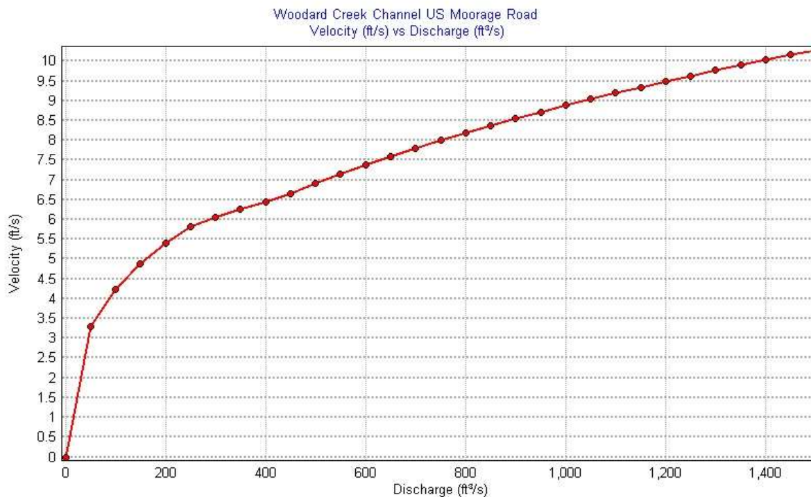
Figure 16. Woodward Creek Reach 2: Velocity and Discharge Rating.
